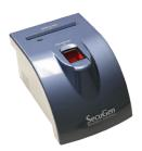
Combination fingerprint reader and contact smart card reader
