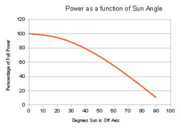
Graph showing the relative power collected by a solar module as a function of the angle relative to the sun. Facing directly toward the sun (0 degrees) is taken as 100% of possible power. Note that a module perpendicular to the sun (90 degree) receives only reflected light which is about 10% of maximum.
