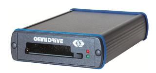
OmniDrive Professional is an external drive for various types of memory cards complying with the memory card standard. This includes SRAM cards, Linear Flash cards, ATA Flash cards, CompactFlash cards, ATA hard disks, SmartMedia cards, MultiMedia cards and SD memory cards.
